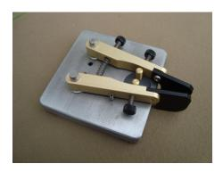
The pin retainer will fit snugly over the tops of the dowel pins. Making sure it is perpendicular to the base, push the retainer down until it bottoms on the base.
