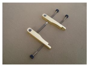
Drop the Delrin disc into the bore in the right lever, and put the closed end of the spring into the bore on top of the washer. With the contact screw fully retracted into the lever, slide the assembly over the right hand dowel pin, making sure the lever is INSIDE the spring pin lever stop. (The lever is between the pin and contact post.)
