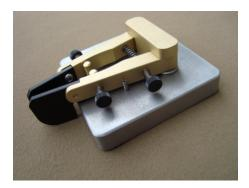
Turn the base over & screw the 6-32 x  $\frac{1}{2}$  screws into the pin retainer thru the base. The ground lug goes under one screw & the cable clamp under the other. Press the sticky-back rubber feet onto the bottom of the base - that's it!
