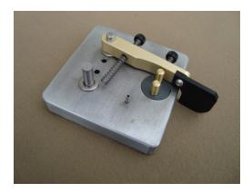
Place the left lever over the left dowel pin so that the lever rests on TOP of the spring pin. Guide the end of the spring into the bore in the lever.
