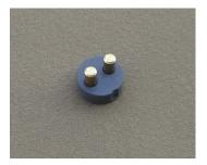
Now turn the insulator over & insert the two 4-40 x 3/16 screws with the #4 terminal lugs into the holes in the bottom of the insulator and thread them into the contact posts. Tuck the contacts together and snug the screws enough to hold the terminals in place. The contacts are pointing away from the notch milled into the edge of the insulator.
