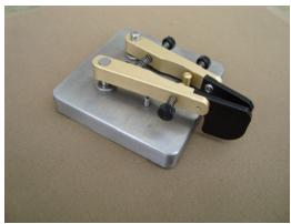
With the spring in place, rotate the lever to the right until it drops in between the spring pin & contact post.
