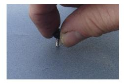
Screw the thumb screws into the sides of the levers, just a few turns. The screw without a ground end goes in the hole in the right lever next to the dowel pin hole.
